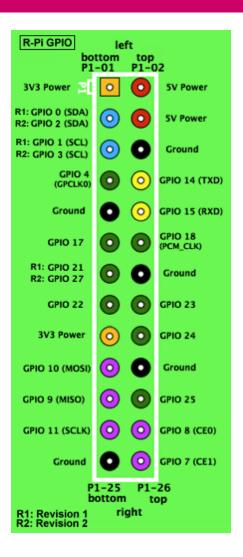
These pins are a physical interface between the Pi and the outside world. At the simplest level, you can think of them as switches that you can turn on or off (input) or that the Pi can turn on or off (output). Seventeen of the 26 pins are GPIO pins; the others are power or ground pins.
