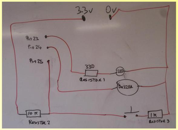
When a GPIO pin isused as an input it is "floating" and has no defined voltage level.
