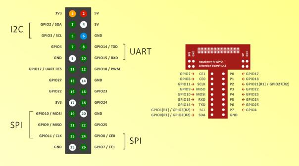
First we need to set up the GPIO pins
